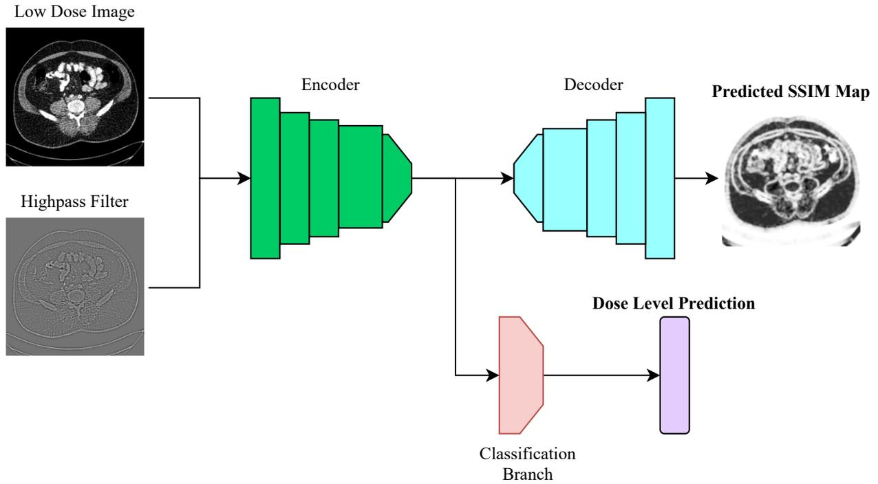
Figure 1. Schematic of the proposed N2Q model. A high pass filter of the input LDCT image is calculated and concatenated with the input image before passing to the model. The model predicts the SSIM map for local IQA as well as self-supervised dose level prediction, which is performed through the classification branch.
